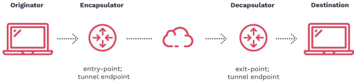
Figure 2.1: Illustrating tunneling
